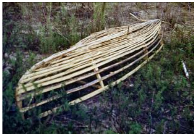
Figure 12. Frame for a birchbark or skin canoe (PWHNC 1979-062-0210)
